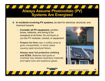
Always assume photovoltaic, or PV, systems are energized, whether or not the sun is shining.
